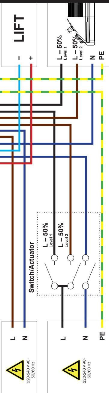
Required wires (acc. to DIN/VDE 0100-520 minimum requirements)
